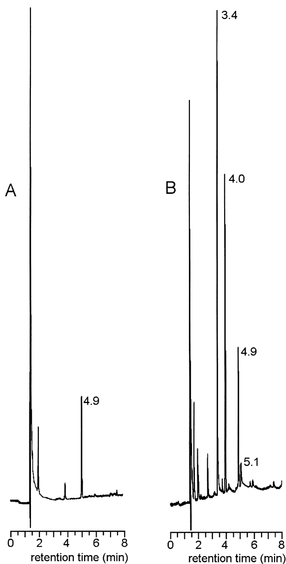
Fig. 4. GC chromatogram of a urine sample, collected prior to (A) and after 6 h of drug administration on day 1 (B). ThioTEPA (4.0 min), TEPA (3.4 min) and monochloroTEPA (5.1 min) concentrations were 587, 1825 and 82 ng/ml, respectively.
